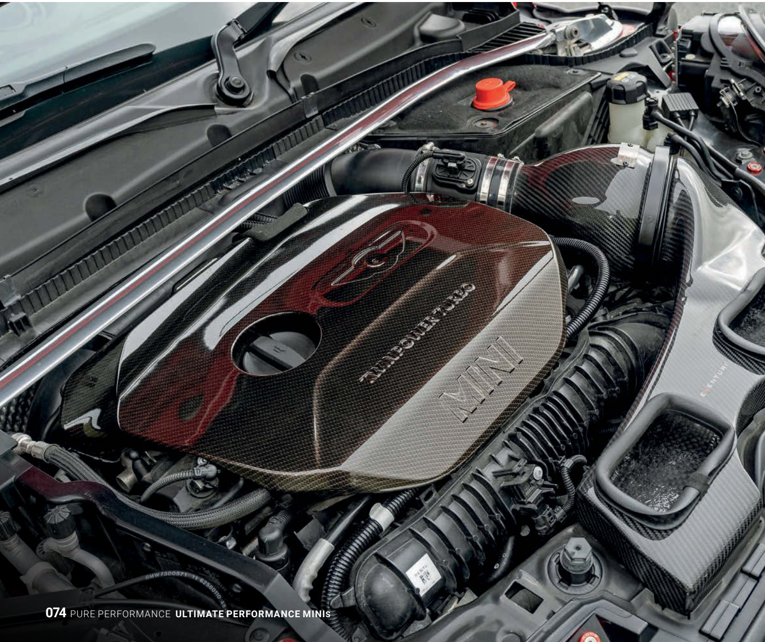
Strut brace is just one of the track-inspired handling upgrades on this JCW
